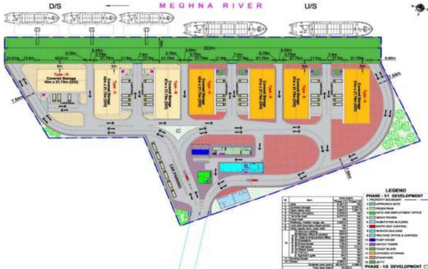
Figure 76. Ashunganj Terminal final Design
